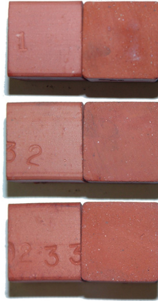
Figure 6. Fired bars, cross-sections.
